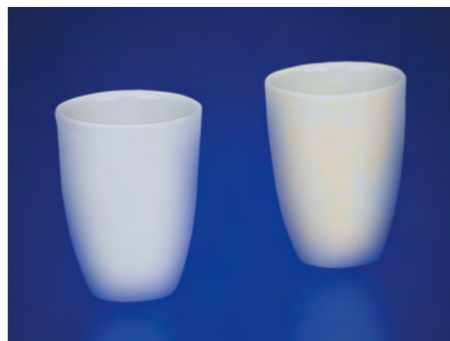
Competitor crucibles shown before (left) and after (right) anneal testing. Significant discoloration can be detected after the first anneal cycle.
